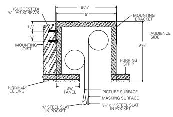
Offset mounting, recessed above ceiling. May be adapted for 1/4" paneling for ceiling.
