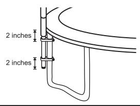
6. Feed the screw through the screw hole thus tightening the clamp to securely connect it to your trampoline leg with the tool included.
