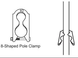
3. Once the pole is securely inserted into the clamp you can now clasp the leg into the larger hole of the clamp. Making sure that the black rubber cap of the lower pole faces down.
