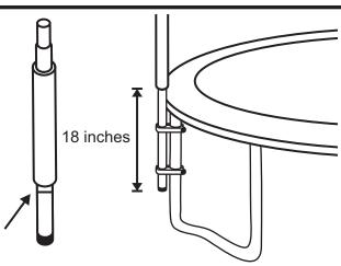
**5**. The set comes with 2 clamps per pole. One being attached 2" **below frame**, while the other being attached 2" **above the end of the lower pole**.
