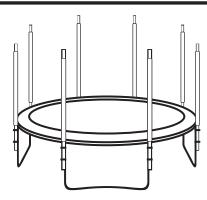
**9.** 9. After connecting all Enclosure Poles insert the Pole caps, if you have an Inside Type Net use part number E1 and for outside type Net use E2
