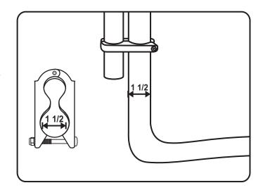
**Note:** You can also connect the poles to the leg with U shape connecter Model UBHWD-UB-12 for set of 12 and model UBHWD-UB-16 for set of 15.
