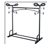
Place the 2 K-3 Cradles (Part D) onto the lower Vertical Post (Part C), and connect the Horizontal Arched Beam (Part E.) with 4 long screws (Part I)
