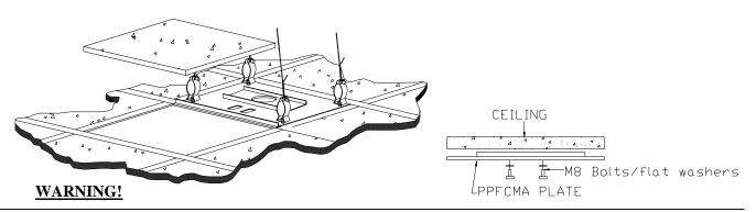
The ceiling should be capable of supporting a weight of at least five times the projector or monitor weight. If it cannot, the ceiling must be reinforced. Proper installation procedure by qualified personnel as outline. In the installation instructions must be adhered to. Failure to do so could result in serious personal injury. For further information or ordering assistance contact us at the address shown on the front of this page.
