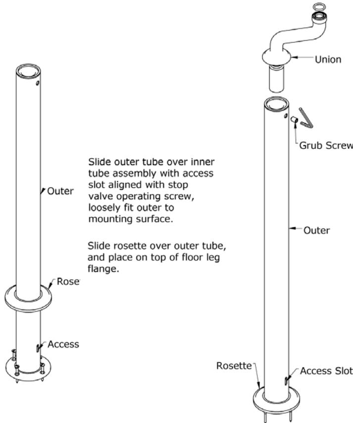
Slide union into outer taking care not to damage sealing rings once union has located on inner tube. Fully secure assembly to mounting surface.
