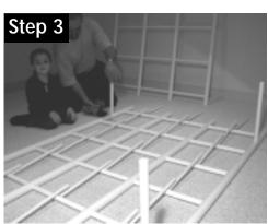
All Horizontal Sliderails fastened to Rear Grid. Now Fasten 4 Front and Rear Grid Connecting Tubes (#5) to Rear Grid using 4 - #06 x 1/2" Fastening Screws (#1)
