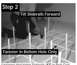
Fastening Horizontal Sliderails (#7) in Rear Grid using 18 - #06 x 1/2" Fastening Screws (#1)
