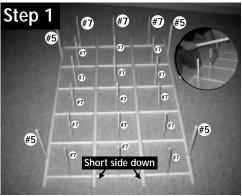
18 Horizontal Sliderails (#7) and 4 Front and Rear Grid Connecting Tubes (#5) inserted in Rear Grid
