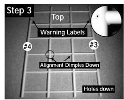
1 Left Front Corner Vertical (#4) and 1 Right Front Corner Vertical (#3) - Placed on Horizontal Crossbars (Holes Facing Down)
