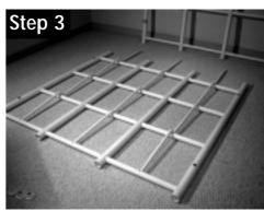
All Horizontal Sliderails fastened to Rear Grid **Note: Fastener in Bottom Hole Only**
