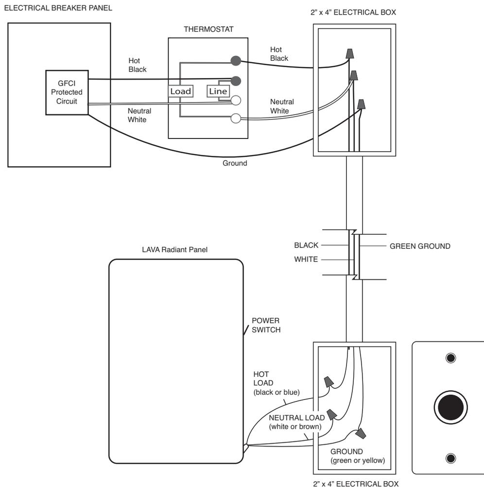
Fig 9: Connection diagram
