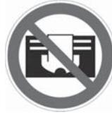
**WARNING:** Covering the glass surface causes overheating danger! May cause damage to the heating element.
