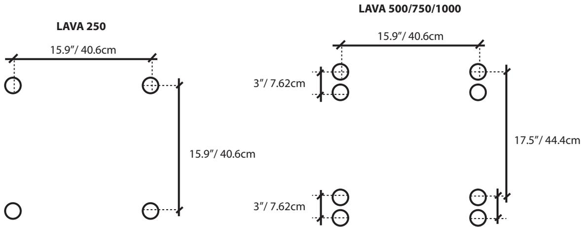
Graphic: LAVA® Glass radiators 250W | 500W | 750W | 1000W - Hole drilling pattern - Wall Mounting
