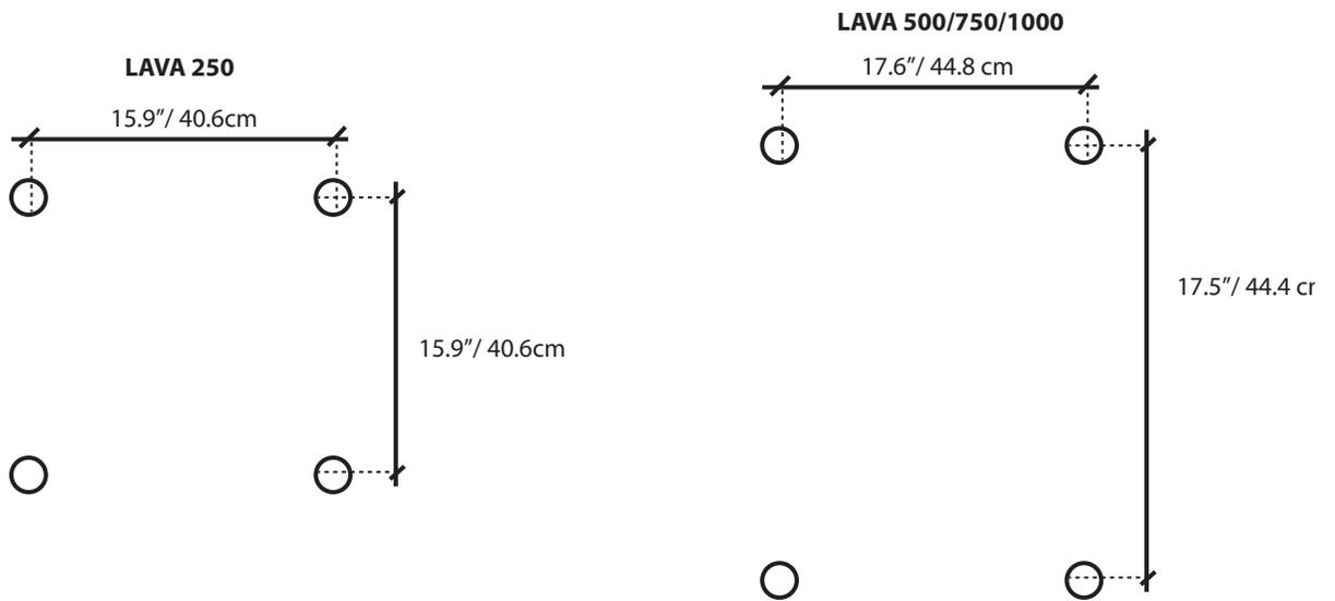
Graphic: LAVA® Glass radiators 250W | 500W | 750W | 1000W - Hole drilling pattern - Ceiling Assembly
