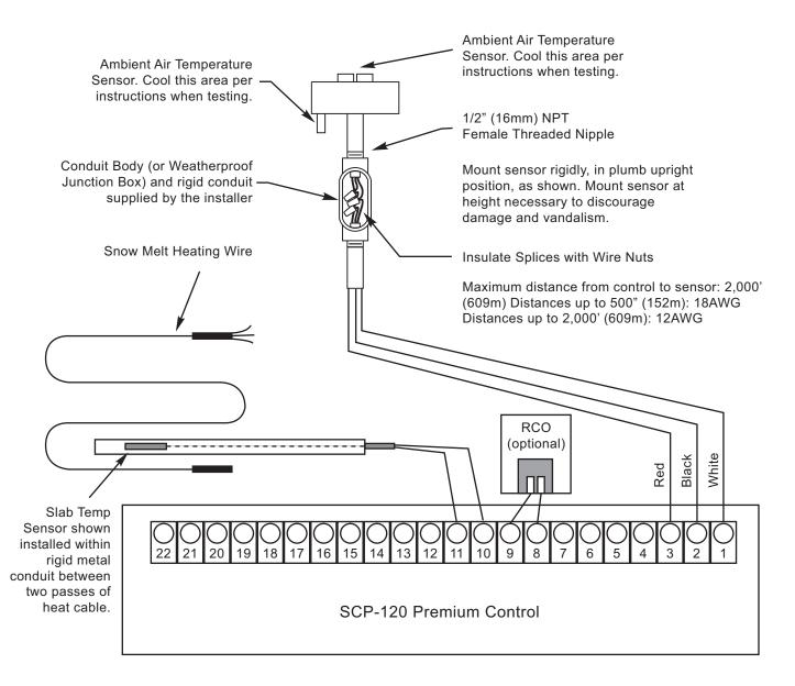
Note: All sensor and remote device connections are low voltage, Class 2 connections
