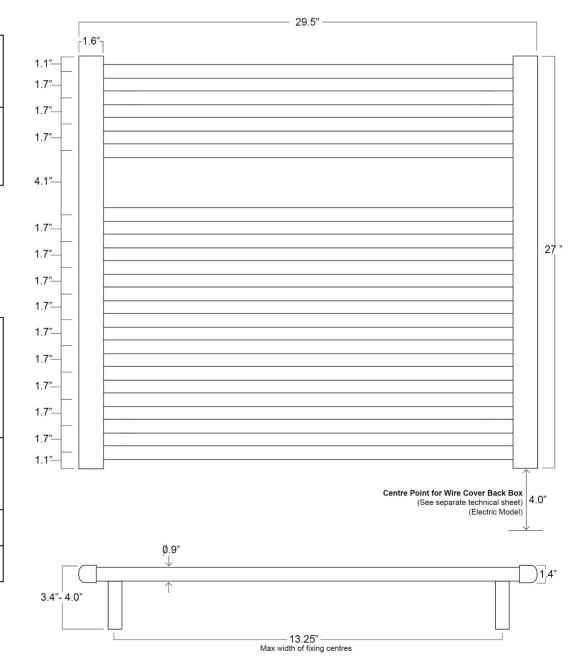
Position mounting brackets as near to each edge as possible and between the first or second cross bars
