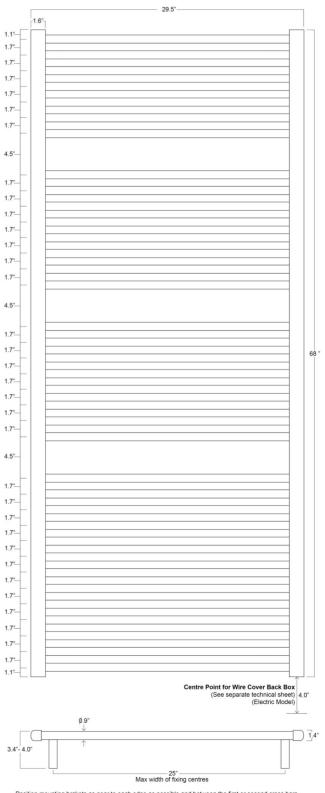
Position mounting brakets as near to each edge as possible and between the first or second cross bars
