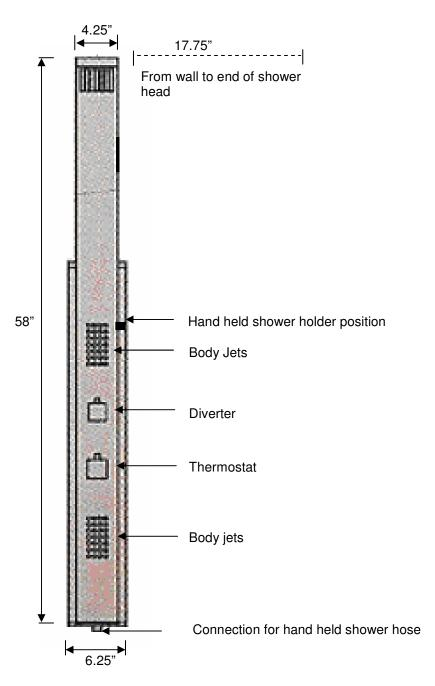
Rough in  $\frac{1}{2}$ " MPT facing upwards max 2.5" centers protruding max 2" from fininished wall surface
