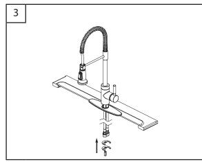
Insert supply hose assembly and thread rod through hole of sink (through center hole of escutcheon if used). Install rubber washer, metal washer and retaining nut onto the threaded rod. Firmly tighten retaining nut. Do not overtighten.
