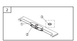
Place base plate (#2) and escutcheon (#1) on the sink. If you have no use for the escutcheon, please use seat (#3) to replace escutcheon and base plate.
