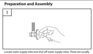
found under the sink or near the water heater. Remove old faucet. Clean and dry sink surface area where new faucet will be mounted.
