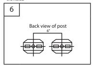
When installing tissue paper holder, center mounting brackets as shown.
