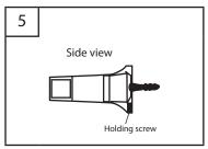
Place base over mounting bracket and tighten the holding screws.
