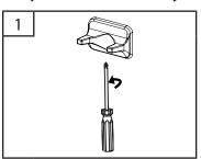
Determine desired location for your new bath accessories. Unscrew set screw at base of each post and remove mounting screws and brackets.
