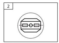
Determine desired location for your new bath accessories. Position base on wall where desired and lightly outline. Center mounting brackets horizontally in outline of posts.
