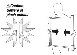
**Note:** Do not touch the screen surface. Handle the MicroScreen only by the case sides or handle.
