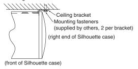
To mount suspended from ceiling, the brackets need to be installed on screen case as noted on page 1. Use "S" Hooks through the holes in the brackets to attach to ceiling. Select the set of holes that allows the screen to hang in a vertical position. The installer is to provide the "S" Hooks and the materials and fasteners to attach the "S" Hooks to the ceiling. Installer must insure that the fasteners and suspension material is of adequate strength and suitable for the mounting surface chosen.
