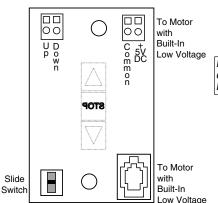
Please Note: 5V DC must be connected to be able to set limits using the wall switch.
