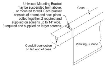
Motor end bracket must be located 1"-6" to right of access door. Idler end bracket must be located 6"-12" from right end of case. Failure to mount brackets as directed could cause the case to bow and result in damage to screen.
