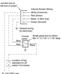
Rolleramics over 12' x 12' have a blue wire lead instead of a black wire lead coming from the motor.
