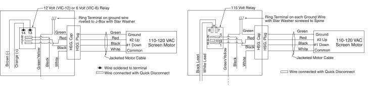
\*These wiring diagrams are for Access screens with motor on audience left (standard), and fabric unrolling from the back of the roller (standard).
