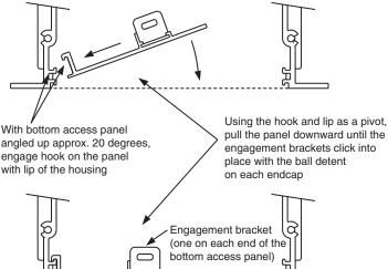
With bottom access panel angled up approximately at 20° it can be lifted off of the lip of the housing and then lowered out of the housing completely.
