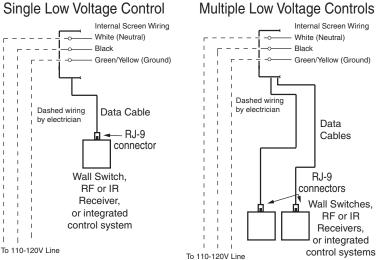
\*These wiring diagrams are for Access screens with motor on audience left (standard), and fabric unrolling from the back of the roller (standard).
