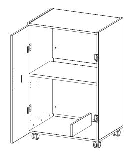
Attach the Right Door (J) using four  $#8 \times 5/8$ " Flathead Screws (H17) in the pre-drilled holes as shown.
