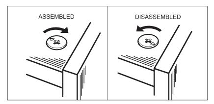
Place the Divider (L) on a clean, carpeted surface with the predrilled holes facing up. Insert two Minifix Cams (H1) into the Divider with the arrows of the cams facing out.
