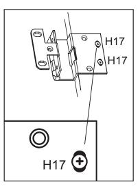
With a screwdriver, attach the Hinges (H6) to the Right Side (B) using the  $#8 \times 5/8$ " Flathead Screws (H17) in the pre-drilled holes. The screws must be centered in the slots
