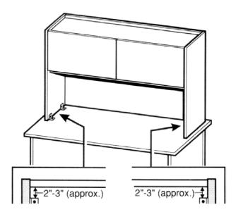
**C.** Using an electric drill and a 1/8" bit, drill the pilot holes 1/2" deep.
