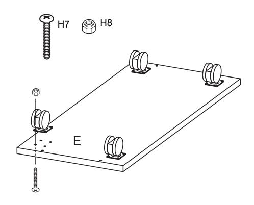
Position Bottom (E) with the caster-side up onto the main assembly. Fasten in place using four #8x50 Confirmat Screws (H3) as shown.
