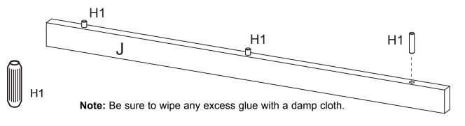
**#2** Glue the Facia Strip (J) to the underside of the Worksurface (C) as shown. Fill each hole 1/4" full of glue and press Facia Strip until fully seated in place. Set aside to dry.
