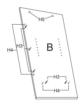
Insert six 19mm Minifix Cams (H5) into the Back Panel (D) and four 19mm Minifix Cams into the Bottom Shelf (D) facing out.
