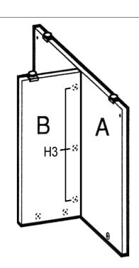
Position the Support Assembly (A & B) onto the bolts and dowels of the Top Panel (C) and turn the Minifix Cams (H3) clockwise to secure.
