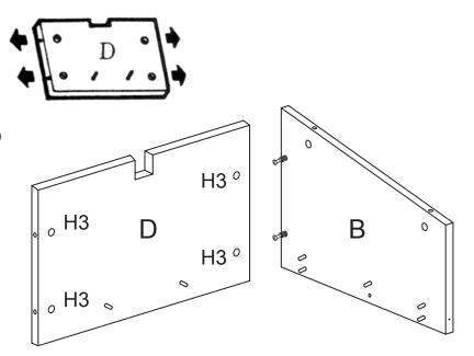
Position the Left Lectern Side (A) posts into the Cam Devices of the Lectern Back (D) and rotate Cam Devices until secure.
