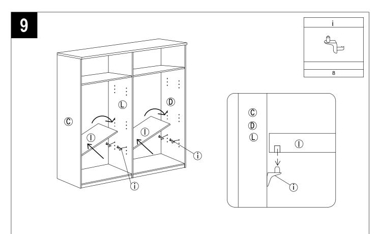
Insert the shelf support (i) into the holes of left / right side panel at the desired height, then
