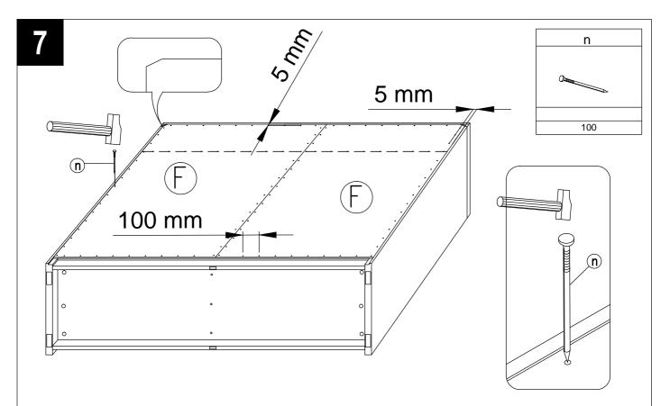
• Position nails (n) 5 mm in from side edge of the back panel with distance 100 mm between each other. Fix them using the hammer.
