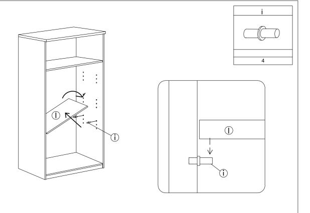
• Insert the shelf support (i) into the holes of left / right side panel at the desired height, then place the shelf (I) onto the support.
