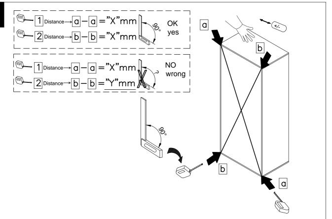
• Before fixing the back panel (F), the diagonal lines must be equal. ("a" to "a" and "b" to "b")
