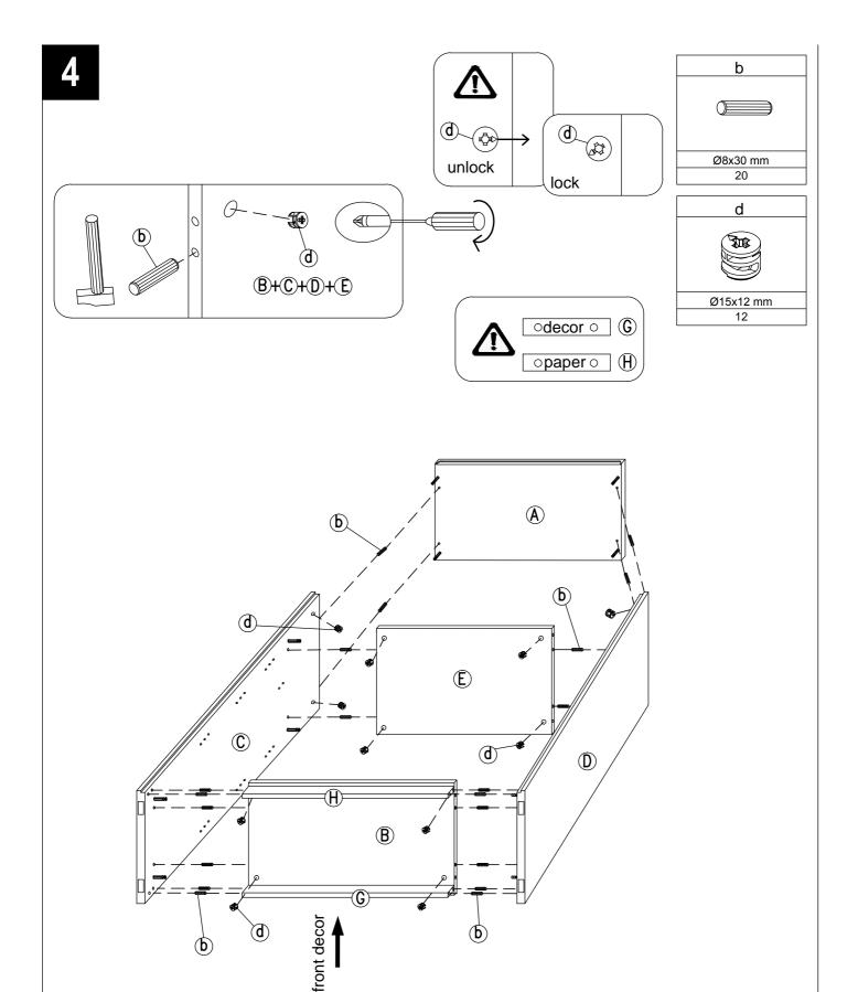
Attach top panel (A), bottom panel (B) and fixed shelf (E) to the left / right side panel (C&D) with wooden dowel (b), then insert cam lock (d) into the holes as pictured on the underside of panels and tighten.
