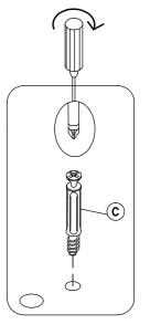
• Fit the cam bolt (c) to the panel (A).
