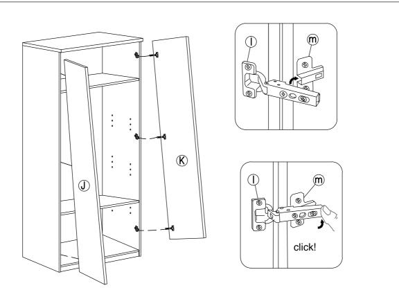
Attach the doors by screwing the door hinge (I) to the door hinge B (m) on left / right side panels.
