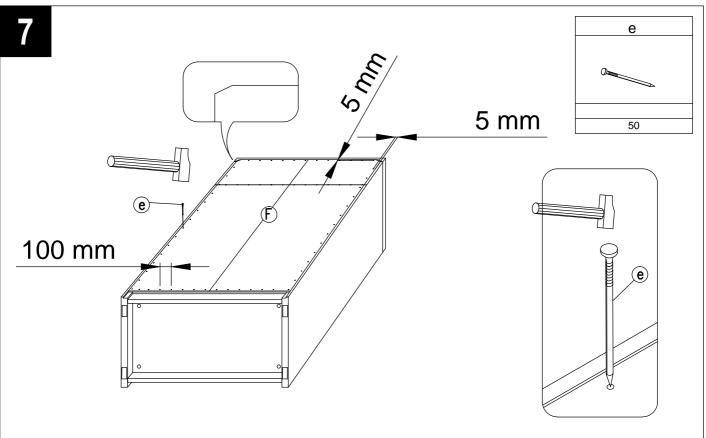
Position nails (e) 5 mm in from side edge of the back panel with distance 100 mm between each other. Fix them using the hammer.
