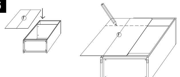
Turn the carcass on the front. Put the back panel (F) between top and bottom panel and draw a line according to fixed shelf.
