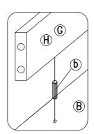
• Attach front plinth / back plinth (G&H) to the bottom panel (B) with wooden dowel (b).
